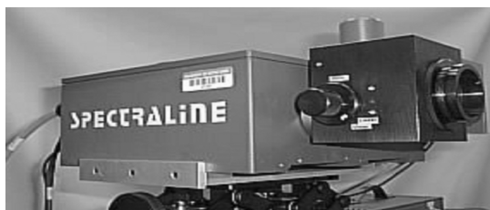
Fig. 2 Photograph of the ES100 spectrometer with the SS100 scanner.
